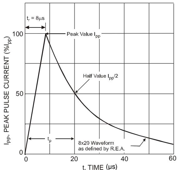
Fig. 2 Pulse Waveform
