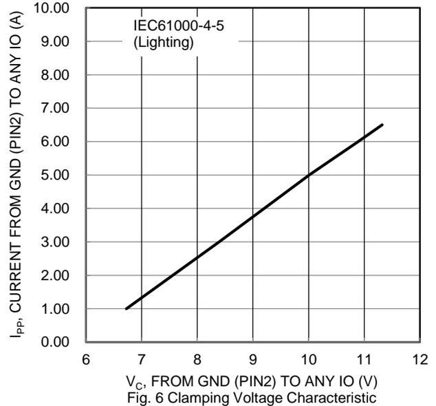
Fig. 6 Clamping Voltage Characteristic
