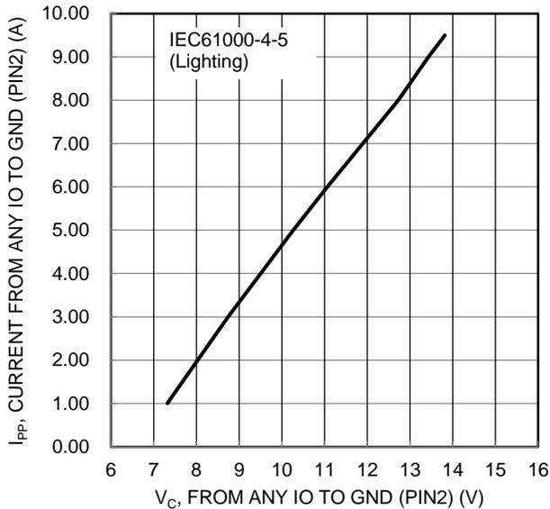
Fig. 5 Clamping Voltage Characteristic
