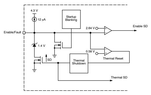
Figure 20. Enable/Fault Simplified Circuit
