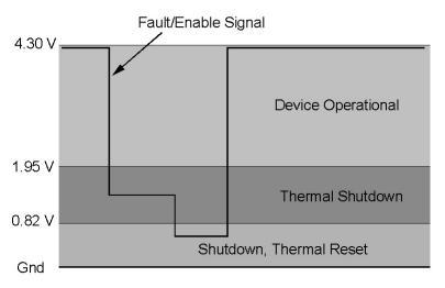
Figure 19. Fault/Enable Signal Levels
