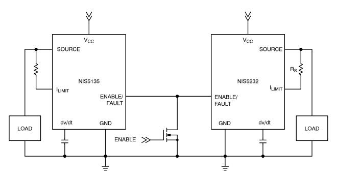
Figure 5. Common Thermal Shutdown
