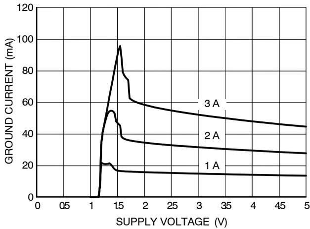
Figure 10. Ground Current vs. Supply Voltage (1.24 V)
