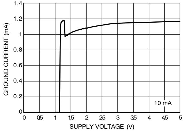
Figure 9. Ground Current vs. Supply Voltage (1.24 V)
