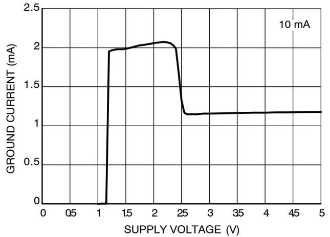
Figure 11. Ground Current vs. Supply Voltage (2.5 V)
