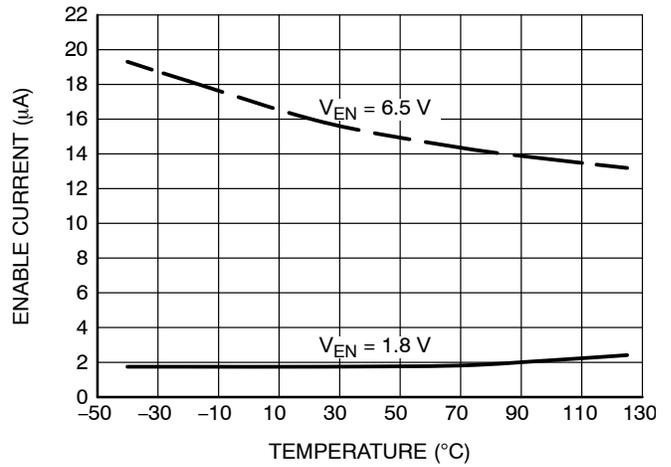
Figure 17. Enable Pin Input Current vs. Temperature
