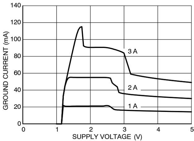
Figure 12. Ground Current vs. Supply Voltage (2.5 V)
